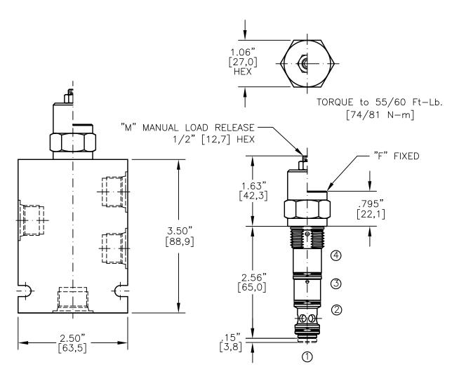
NOTE: CAVITY BOTTOM HOLE MUST ALLOW FOR POPPET EXTENSION (.563 DIA.). FOR ALUMINUM OR STEEL VALVE HOUSING CONFIGURATIONS SEE PAGE 0-042-1.
